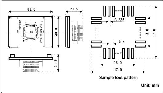
Figure 5.4 External dimensions of the FLX-120NSE
